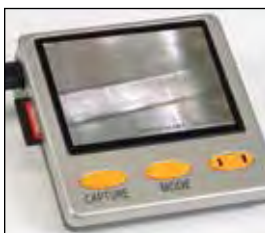
Images can be captured from the display and saved to a memory card.
