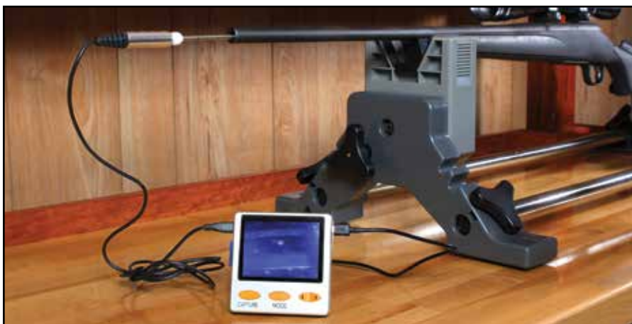
Images can be captured from the display and saved to a memory card.
