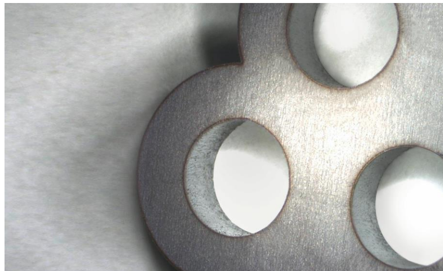
Fig.: Cut parts made of various metals and alloys with nearly any contours can be made with the LPKF PowerCut precision laser system.
