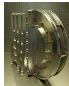
Fig. 1 ENA instrument on BepiColombo / MMO
