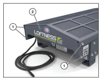
While the oil cooler is still on the ground remove the four bolts (1) securing the back cover (2) to the cooler frame.
