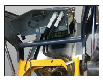
Make sure the hydraulic hoses are routed as shown above. Tighten all connections.
