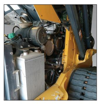
Lift the rear engine compartment door up and remove the right and left side engine panels. Refer to the John Deere track loader owner's manual for instructions.
