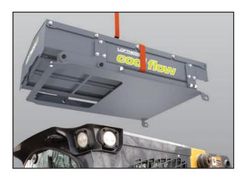
Carefully lift the oil cooler cab mount kit onto the cab of the track loader.
