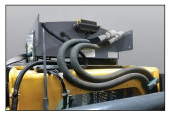
Make sure the oil cooler hydraulic hoses and wiring harness are secure. The hydraulic hoses and wiring harness coming from the oil cooler should route as shown above.
