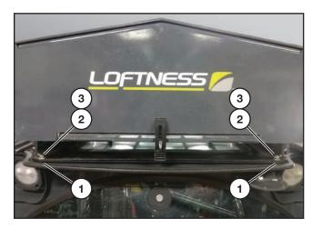
Lower the front of the oil cooler down onto the cab.
