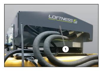
Reinstall the back access cover (1) onto the oil cooler and tighten the bolts.
