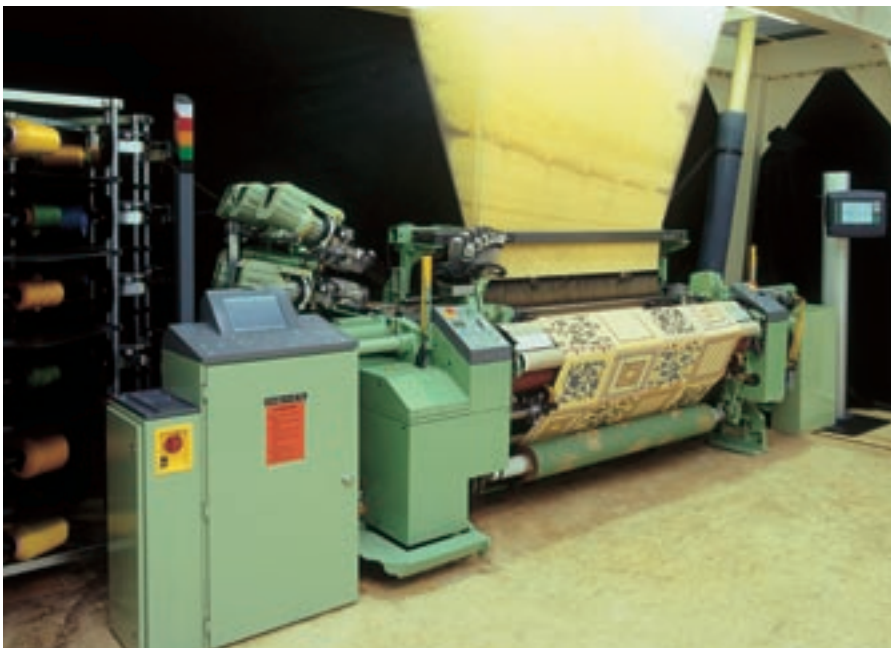
Rapier weaving machine, type PS, in 180 cm nominal width, 12 colors and Jacquard machine with 10,780 lifting hooks
