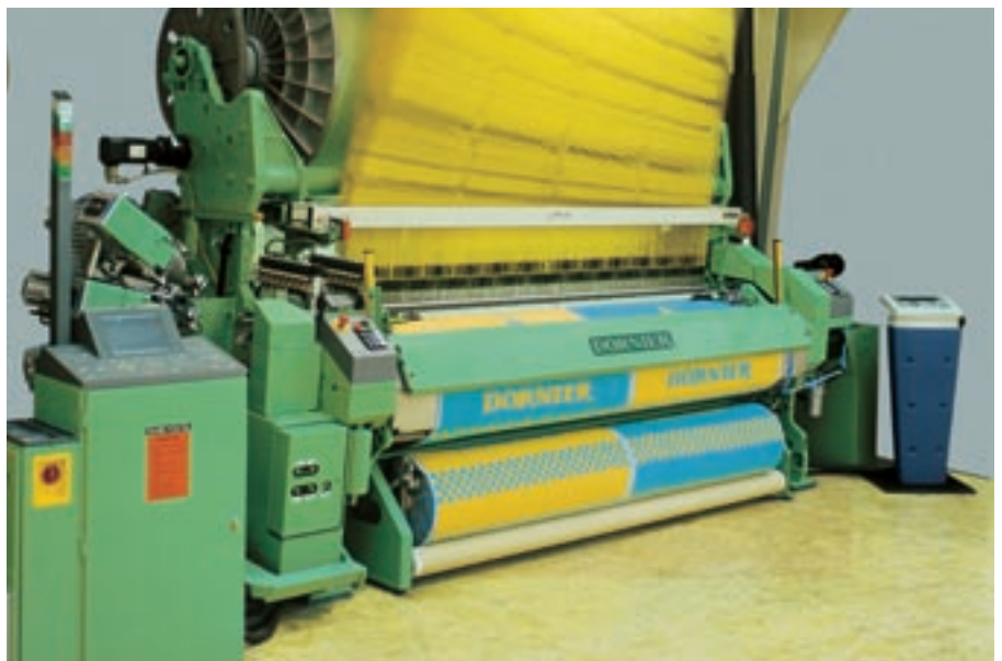
Air-jet terry weaving machine, type "ServoTerry®" with 8 colors in Jacquard version
