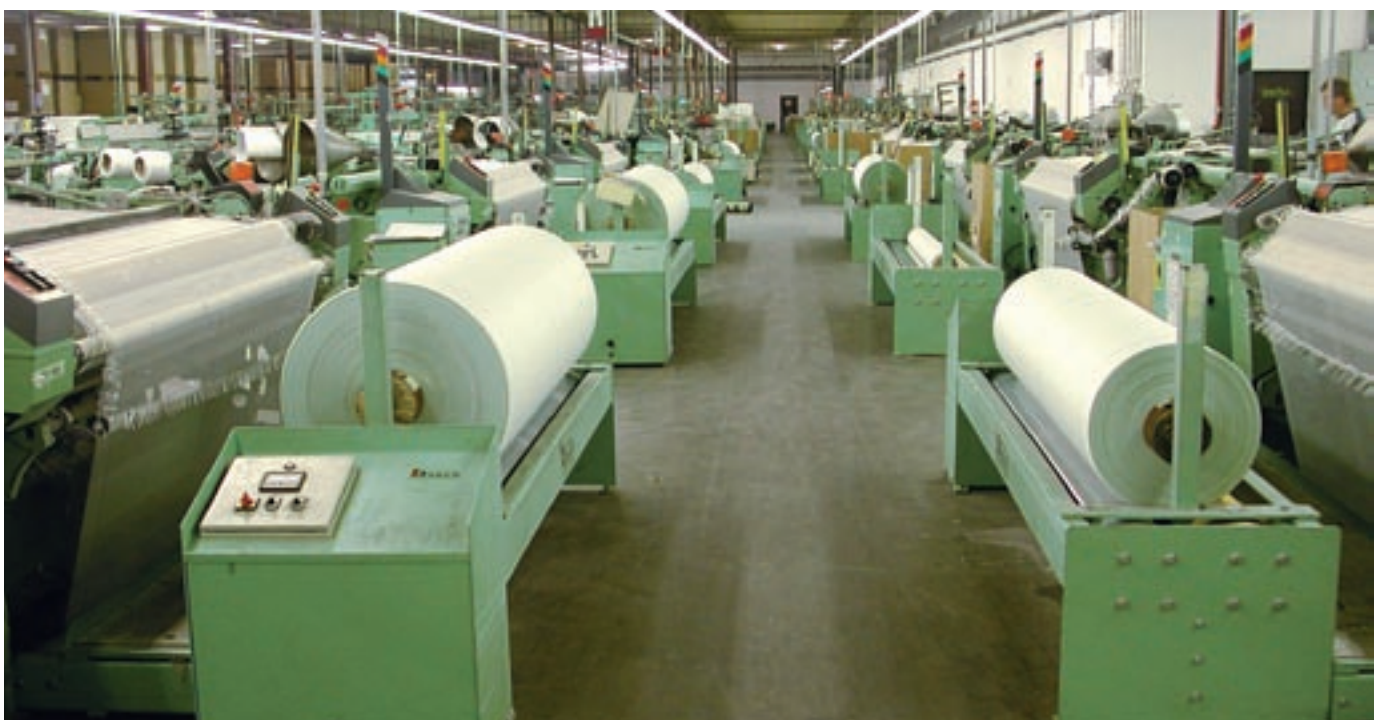
DORNIER rapier weaving machine plant with new EasyLeno®-system for glass leno fabric in Slovakia
