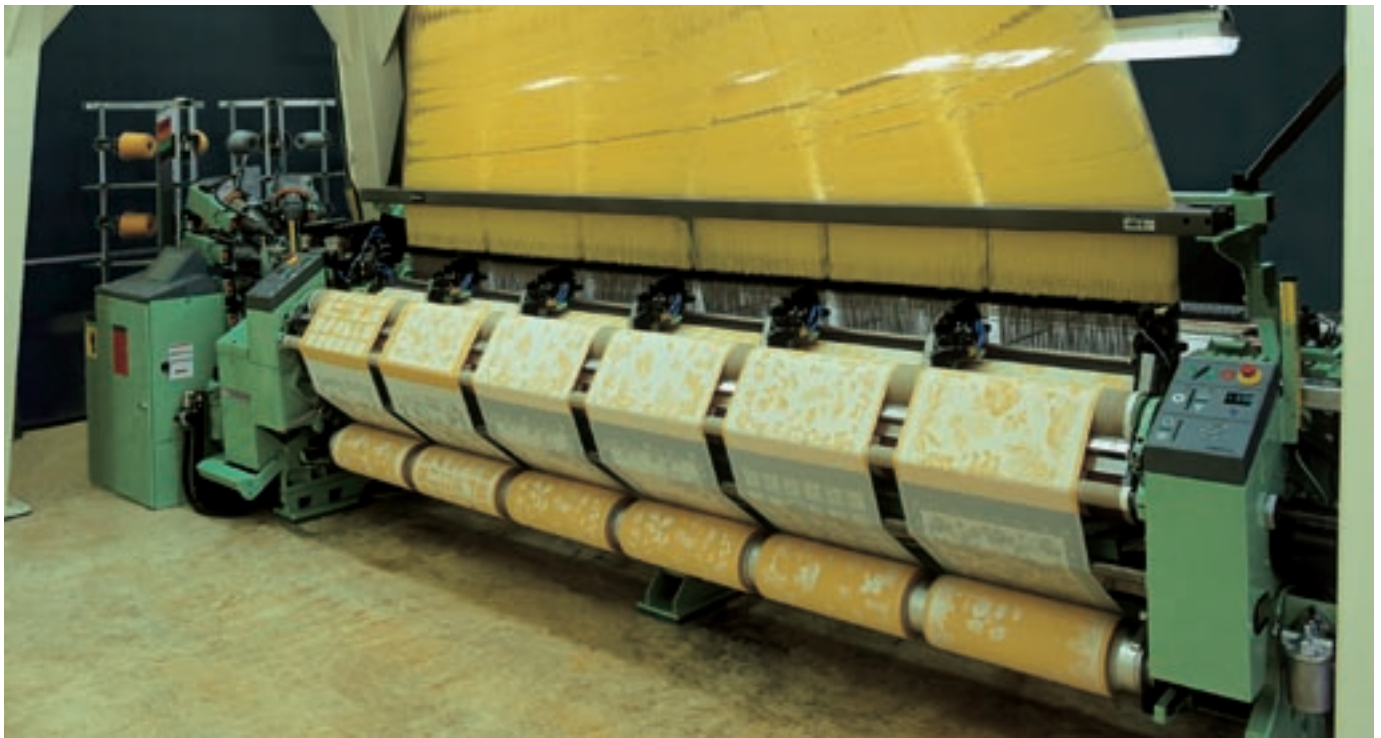
Air-jet weaving machine , type AS, in 360 cm nominal width with 8 colors, pneumatic outer and center tuckers, type PneumaTucker® and Jacquard machine with 10,400 lifting hooks
