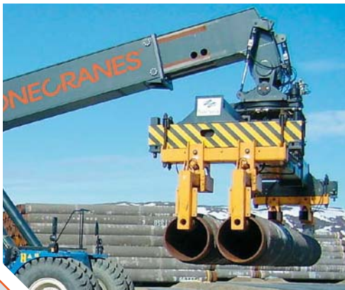
Lift unit for pipes/tubes.
