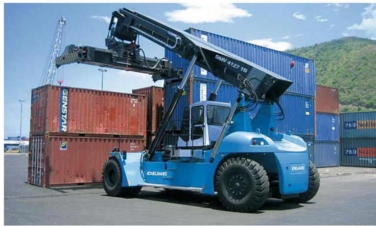
A hard worker that's ideal for terminals where the pace is high. Our big trucks are well-equipped flexible machines. Lift 41 - 45 tons, up to 5 or 6 containers high.
