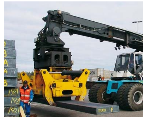
Lift unit for steel slabs and coils.
