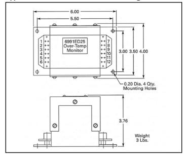
Catalog No. 6991ED25 supersedes and is interchangeable with Overtemperature Monitor Catalog No. 6999ED207C2.
