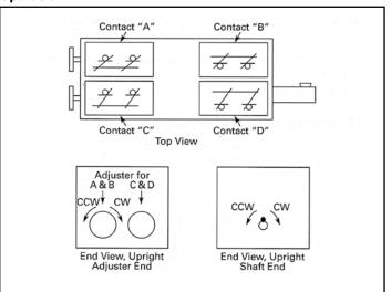
All contacts are closed between limits, the switch construction is such that contact "A" and "D" are normally open before they are mounted in the switch, and contacts "B" and "C" are normally closed before mounting in switch.
