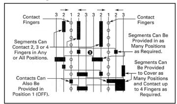
② Diagram for 5-position reversing selector switch showing typical contact segment combinations which are available.
