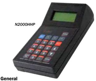
The N2000 Hand Held Programmer (N2000HHP) is designed to facilitate the setup of any of the various styles of the N2000 Overload Relay. The N2000 Overload Relay family contains many programmable motor protection and control features. The N2000HHP is able to access and modify all of the programmable features of the N2000 Overload Relay. These features may be accessed directly via the function select keys, or indirectly by means of stored setups.
