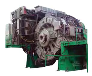
Specifications: 36.5 MW PM **Machine for Electric Ship Propulsion**
