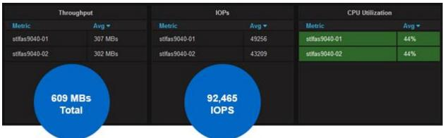
Figure 68) Average CPU utilization, throughput, and IOPS for a FlexGroup volume—AFF A700 HA pair, 128 threads.
