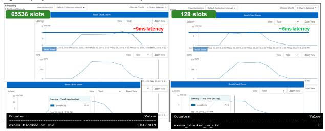
Figure 42) Impact of RPC slot tables on NFSv3 performance.
