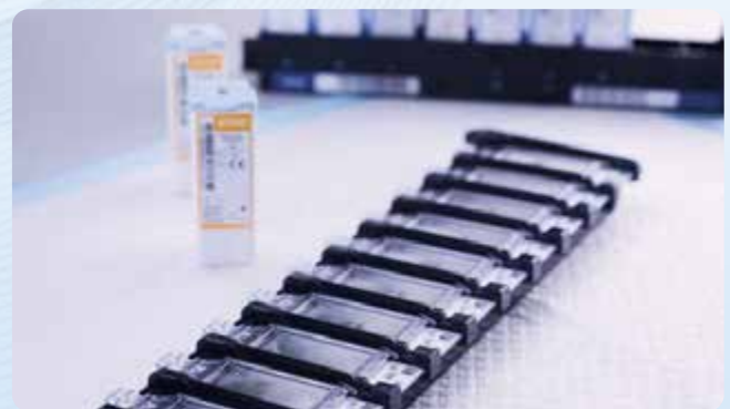
BOND Universal Covertile facilitates gentle, even reagent flow over tissue
