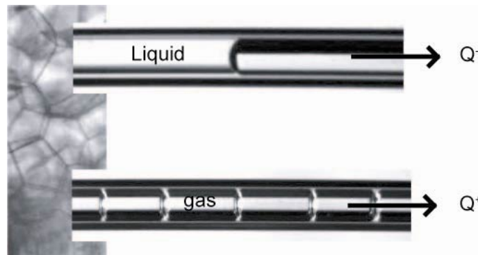
Figure 1 : Foam suction through a capillary tube for different suction flows
