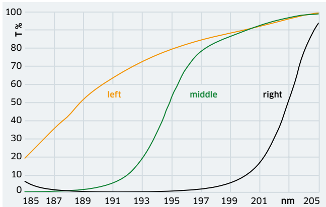
GOC 193 nm/0° [B-00810] 193 nm: right → left position; T = 1% → 70% (MS-coating)
