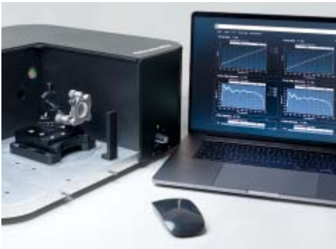
Custom-built white light interferometer
