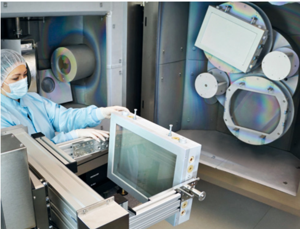
“Teresa”, the largest IBS machine, suitable for substrates up to \varnothing 550 mm
