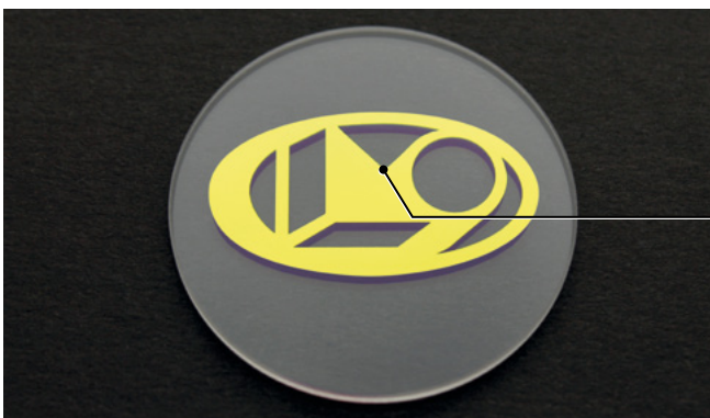
Our logo on a \varnothing 50 mm substrate, showing the shape's accuracy
