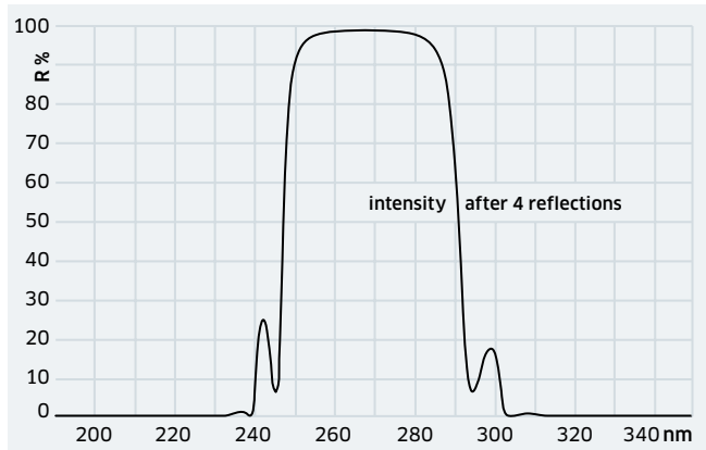
REF 266 nm/45° Type 2 [B-04555] 266 nm: R^4 > 95\% , compensation of manufacturing tolerance for wavelength by angle tuning necessary
