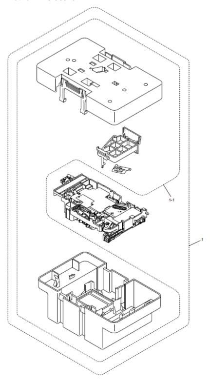
1 <u>D006S7001</u> 1 HEAD/CARRIAGE UNIT (SP) EXCEPT FOR HL-T4000DW/MFC-T4500DW 1 <u>D00STP001</u> 1 HEAD/CARRIAGE UNIT (SP) HL-T4000DW/MFC-T4500DW 1-1 <u>D006VP001</u> 1 PROTECTOR SUPPLY ASSY
