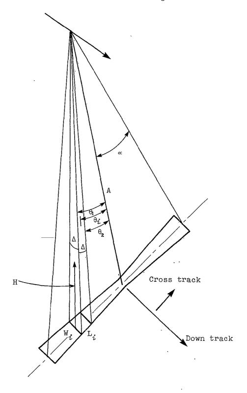
Figure 1. The MSDS ground coverage for one scan line
