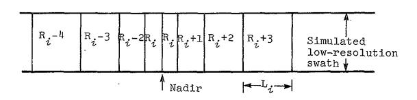
Figure 2b. MSDS samples represent increased ground coverage at off nadir look angles
