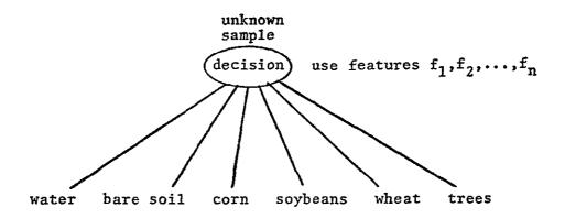
Figure 2.1-1 · Common single-stage classifier.
