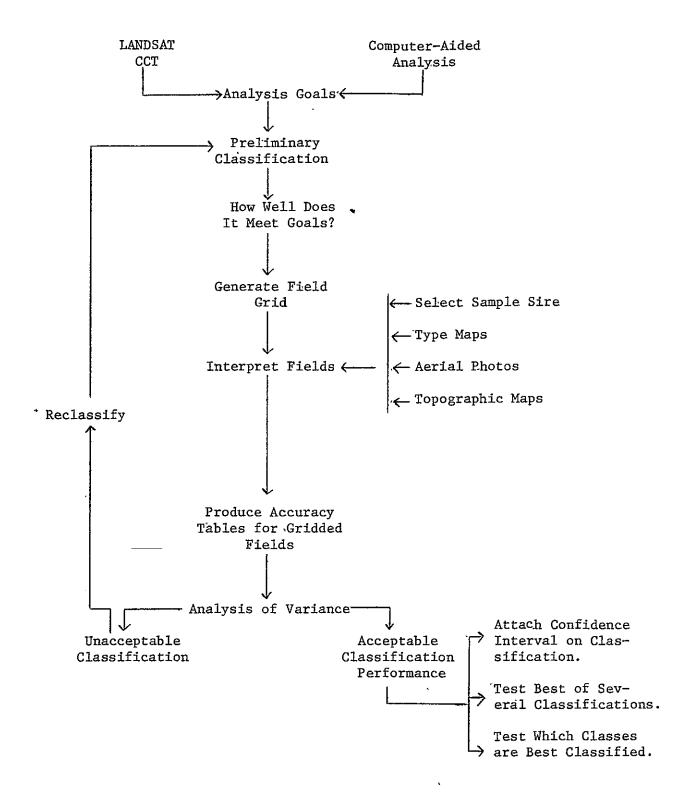
Figure 2.7-1 Steps in Implementing the Stage II Statistical Evaluation Technique
