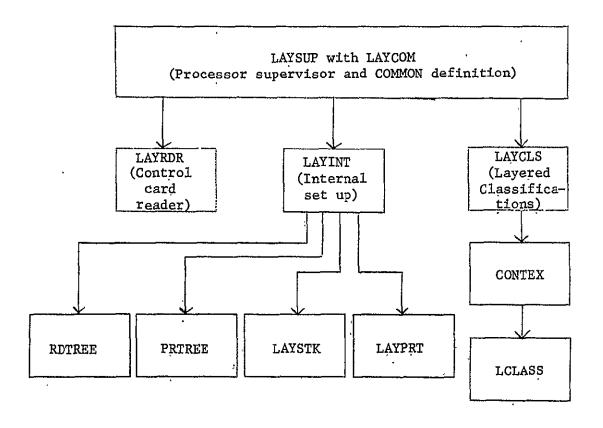
Figure 2.1-7 Layout of the Layered Classifier
