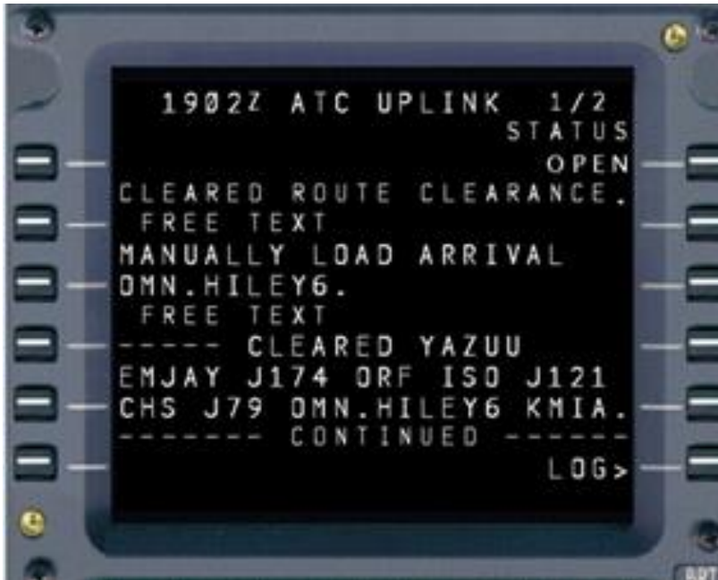
Figure 8 – UM80 Full Route Clearance with Free Text Arrival Procedure and Free Text Modified Route (B737 MCDU Test Bench – FAA Tech Center)
