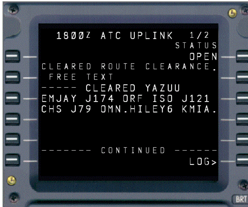
Figure 7 – UM80 Full Route Clearance and Supplementary Route Free Text (B737 MCDU Test Bench – FAA Tech Center)
