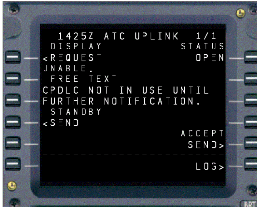
Figure 3 – CPDLC Not In Use Message with an Active Connection (B737 MCDU Test Bench – FAA Tech Center)
