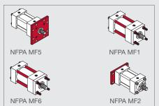
The flange mount is one of the strongest, most rigid methods of mounting. With this type of mount, there is little allowance for misalignment. When long strokes are required, the free end opposite the mounting should be supported to prevent sagging and possible binding of the cylinder. When the cylinder is used in a thrust load application, a blind end flange should be used. For tension applications, rod end flange mounts should be used.
