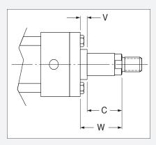
**To Compute:** W = (Stroke x Min. Length Factor) + 1%"
