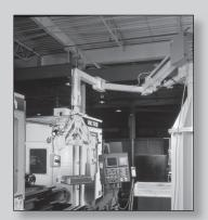
Parts are selected from pallets and moved to working stations. The smooth, positive hydraulic control of the Pow'r Reach™ permits picking and positioning of expensive parts safely and precisely.
