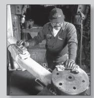
In automated forging processes, hot metal blanks are fed automatically into a progressive die. Each die segment may weigh several hundred pounds and must be handled quickly, easily and safely.
