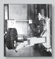
Large and complex cutters are often impossible to handle without some mechanical assistance. The Pow'r Arm™ was adapted for this specific application.
