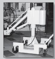
Portable dolly-mounted Pow'r Reach™ provides flexibility to accommodate a wide variety of applications. For stability, a counterweight is welded to the column of these models.
