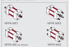
When using tie rods extended on the rod end, the best application is a tension load. For a thrust load application, the tie rods should be extended on the blind end of the cylinder. Tie rod mounts are suited for many applications, but it should be noted that they are not as rigid as flange mounted cylinders and often require additional support for long stroke applications.
