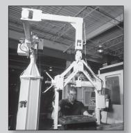
A Pow'r Reach™ is used to position parts in machining centers. It is useful and effective because of the ease and convenience with which the heavy parts are handled.
