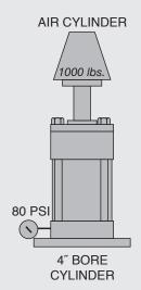
The exact speed of an air cylinder cannot be calculated. Air cylinder sizing depends on the degree of overpowering to move the load, valving, piping, and other factors which usually are unknown and cannot be measured. For further information on air cylinder sizing and speed, refer to page 100.
