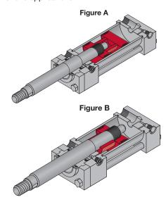
The stop tube is located between the piston and the rod end cap. It limits the extended stroke of the cylinder, providing additional strength for less cost and reduced weight than the use of an oversize rod.
