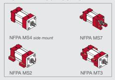
The side or lug mounted cylinder provides a fairly rigid mount. This type of mount can tolerate a slight amount of misalignment when the cylinder is fully extended, but as the piston moves toward the blind end, the tolerance for misalignment decreases. It is important to note that if the cylinder is used properly (without misalignment), the mounting bolts are either in simple shear or tension without compound stresses.
