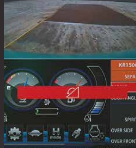
Stability warning display
