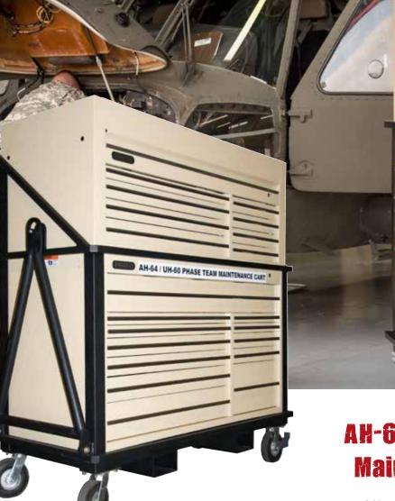
The PTMC consists of 799 items but is not limited to the following; drive sockets, assorted crowsfeet, torque adapters, sheet metal tools, drills, files, snips, pliers, torque wrenches, spring scales, battery operated vacuums, a multi meter, a soldering iron, larger drive sockets, full assortment of stubby and spline drive ratcheting wrenches, screwdrivers and remote area lighting.
