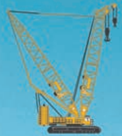
◦ Crawler cranes (55-3600 ton)
