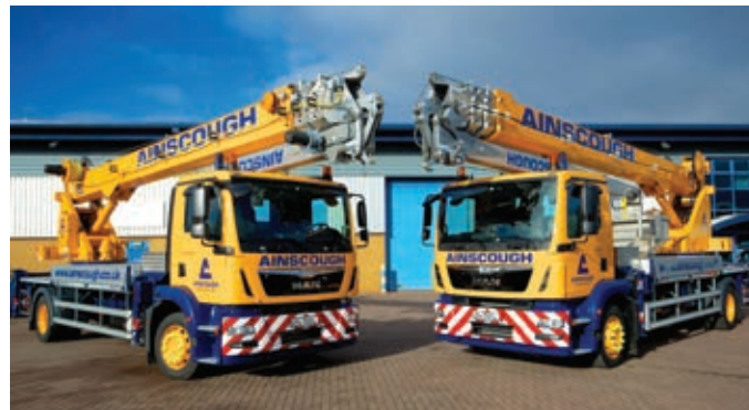
Ainscough's first cranes from German manufacturer Böcker which specialises in building truck mounted units with aluminium telescopic booms
