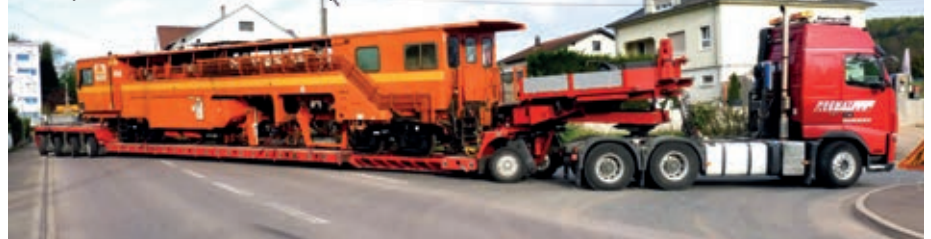
The Nicolas MDEL TP in a 1 + 4 combination being used to transport a rail locomotive to a repair centre
