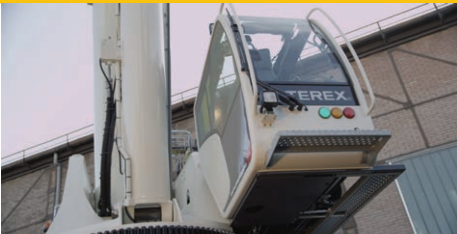
The Explorer 5600 all terrain crane. It was first seen at the ConExpo show in 2014. The 160 tonne capacity model is on a five axle carrier and has all-wheel steering
