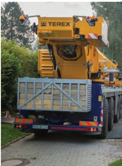
Wooden cribbing neatly boxed on the rear
