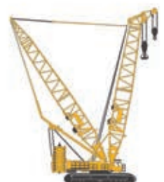
◦ Crawler cranes (55-3600 ton)
