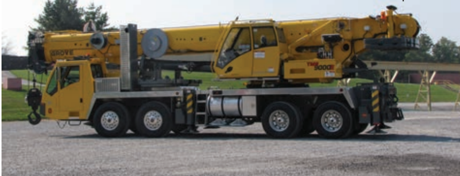
The 90 tonne capacity Manitowoc Grove TMS9000E has an 11.2 to 43.4 m five-section full power boom
