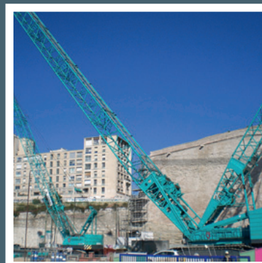
KOBELCO SL6000, 550 ton capacity
