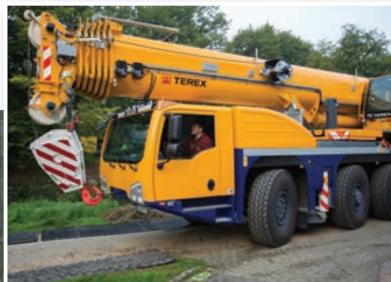
Additional steel plates were placed at the site ready for the crane's outriggers
