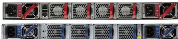
Arista 7050X 2RU rear view: rear-to-front airflow model (blue)
