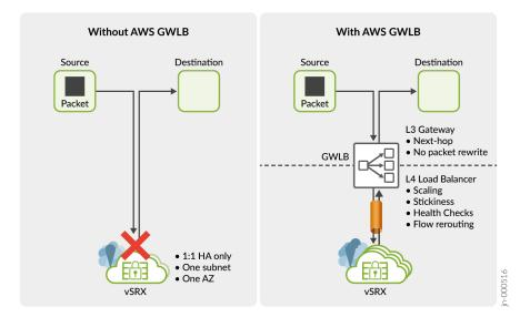
GWLB acts as a Layer 4 (L4) load balancer for the received traffic, enabling you to easily deploy, scale, and manage vSRX Virtual Firewall 3.0. Additionally, GWLB provides stickiness of flows in both the directions. This feature enables vSRX Virtual Firewall 3.0 to see and act on the traffic in both the directions.
