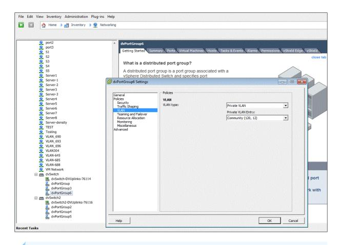
**NOTE**: The configurations described above must reside at an external switch to which distributed switch uplinks are connected. If the link at the external switch supports native VLAN, then VLAN can be set to none in the distributed switch port group configuration. If native VLAN is not supported on the link, this configuration should have VLAN enabled.
