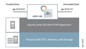
**NOTE**: This example uses static IP addresses. If you are configuring the vSRX Virtual Firewall instance in an *NFV* environment, you should use DHCP.
