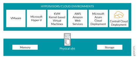
vSRX Virtual Firewall includes the Junos control plane (JCP) and the packet forwarding engine (PFE) components that make up the data plane. vSRX Virtual Firewall uses one virtual CPU (vCPU) for the JCP and at least one vCPU for the PFE. Starting in Junos OS Release 15.1X49-D70 and Junos OS Release 17.3R1, multi-core vSRX Virtual Firewall supports scaling vCPUs and GB virtual RAM (vRAM). Additional vCPUs are applied to the data plane to increase performance.
