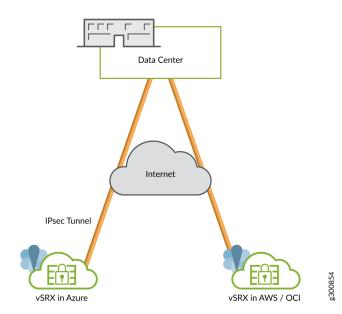
You can generate key pairs using Microsoft Azure cloud HSM service for pkid process and use these keypairs for getting a local certificate from the CA server. Use the keypair present in the cloud HSM service for private key signing during IKE negotiations.
