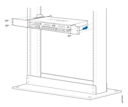
7. Check that the mounting brackets on each side of the rack are level.
