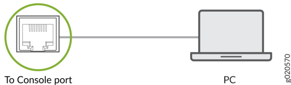
Figure 17: Connecting the MX204 Router Directly to a Management Console
