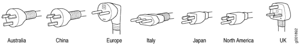
Figure 11: AC Plug Types
