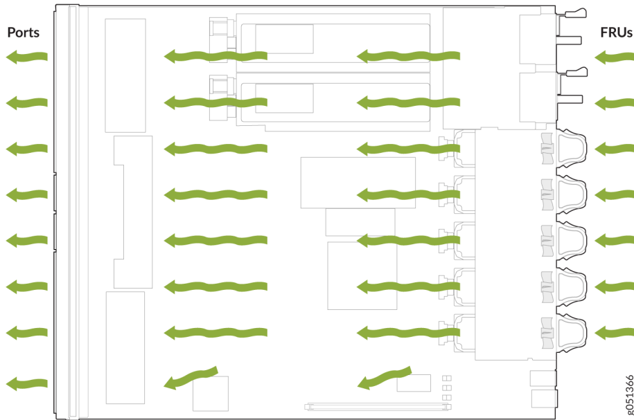
Figure 48: Back-to-Front Airflow Through the QFX5120-48YM Switch Chassis
