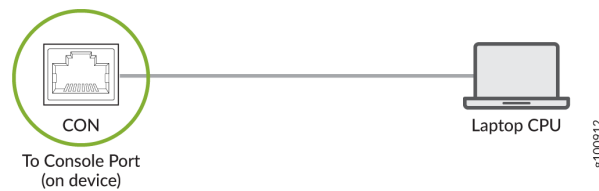
Figure 119: Connect the PTX10008 Router Directly to a Management Console
