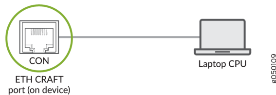
Figure 49: Connecting the PTX10003-80C Directly to a Management Console
