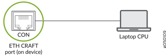
Figure 35: Connecting the PTX10002-60C Directly to a Management Console
