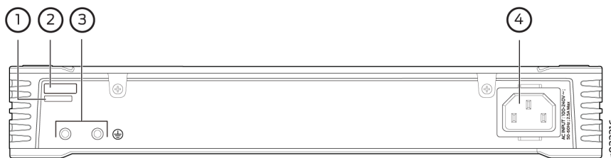
Figure 8: Rear Panel of an EX2300-C Switch with 12 Gigabit Ethernet Ports without PoE Capability
