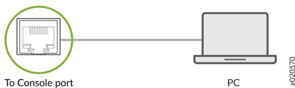
Figure 49: Connect the ACX7348 Router Directly to a Management Console
