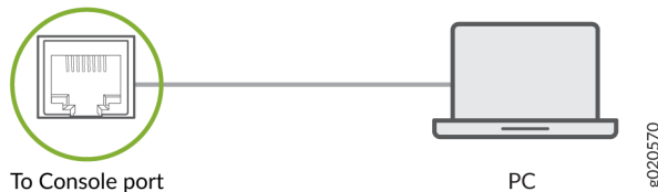
Figure 34: Connecting the ACX7100-48L Router Directly to a Management Console
