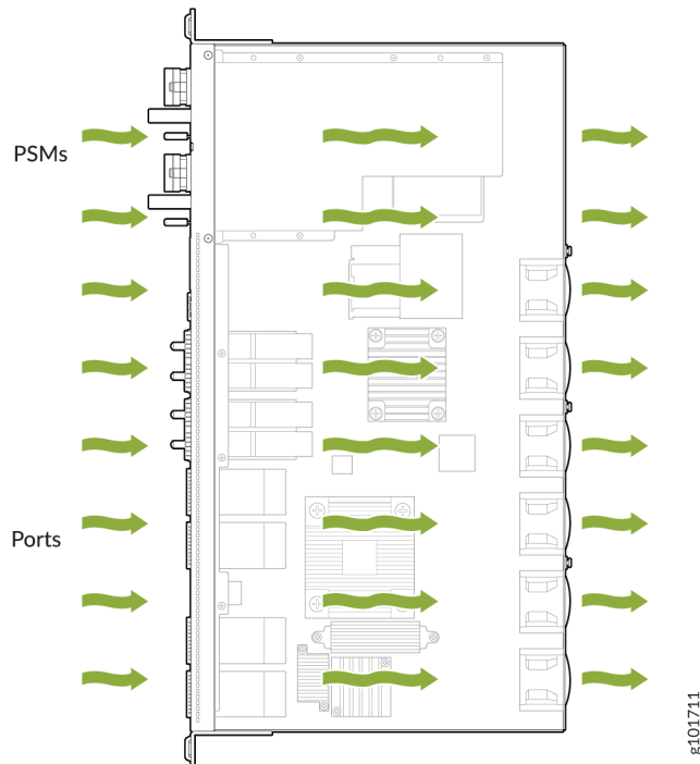
Figure 17: AFO Airflow Through ACX7024 and ACX7024X Chassis
