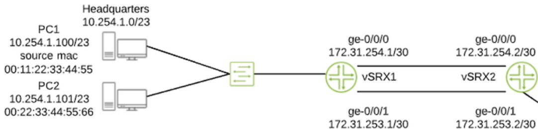
Figure 5.3 Layer 3 Communications from VLAN 1
