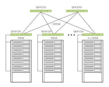
Figure 2: QFX5120 and QFX5210 leaf-spine deployment with distributed gateway
