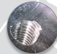
Burr in a cross hole in an ABS brake manifold viewed with a Hawkeye Pro Slim 7"
