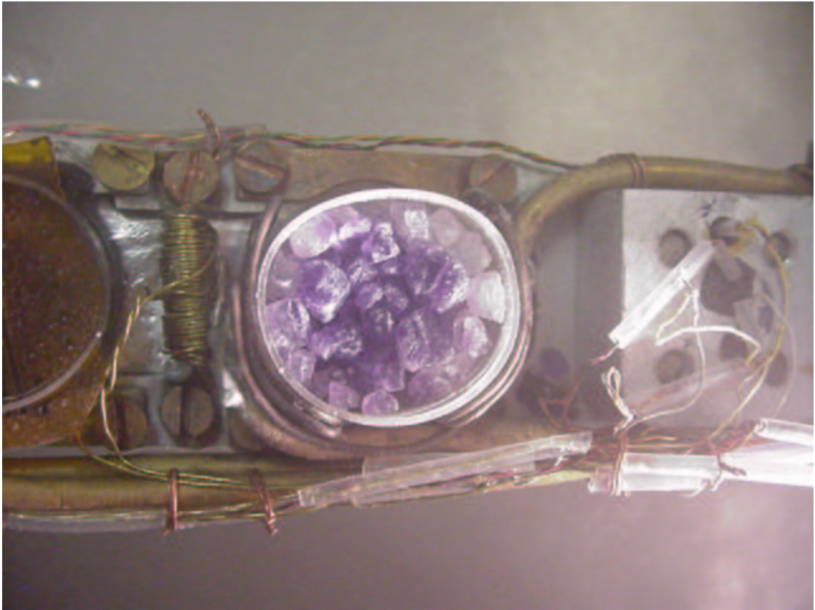
Figure 4.3: A photo of target cell after beam exposure. The beads in the center turn purple from the beam exposure, while the edges do not receive much beam.
