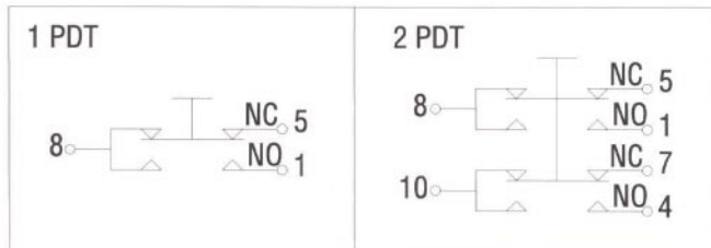
Form "C" Switch Circuits
