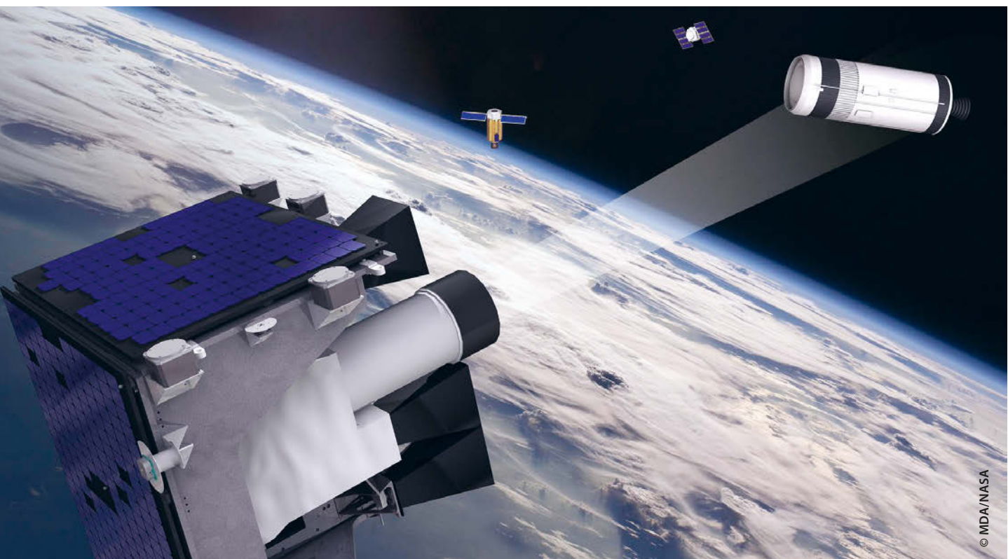
Sapphire is a Canadian LEO small satellite for space surveillance designed to monitor space debris and satellites within an orbit from 6,000 to 40,000 kilometres above Earth. It is operative since 2013.
