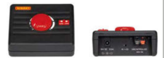
This Analogue Train and Accessory Controller features a sturdy casing, as well as an additional uncontrolled DC output, with integral capacitor discharge unit (CDU) to support solenoid point motors. The Auxiliary output can also be used to power lighting on the layout up to a current of 150mA. A recessed reduction switch also limits the output to reduce loco speed.
