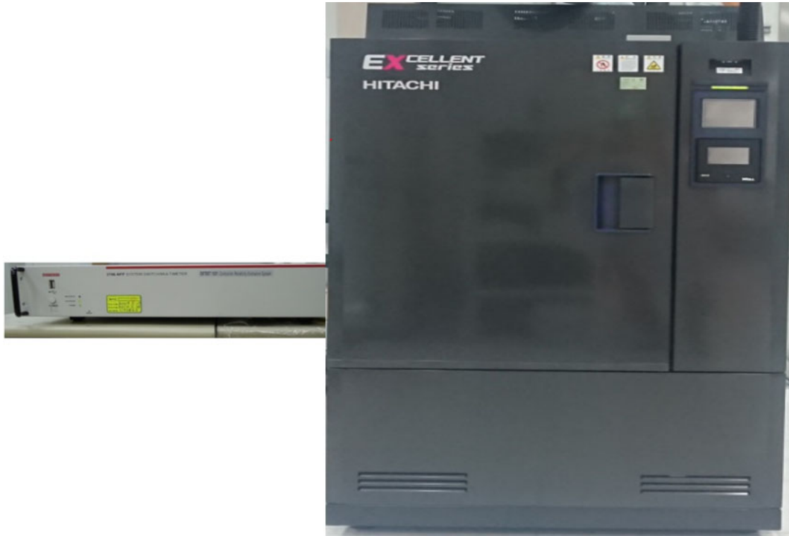
Figure 7. Hitachi Temperature cycle chamber and Keithley system switch/multimeter, for solder joint life test
