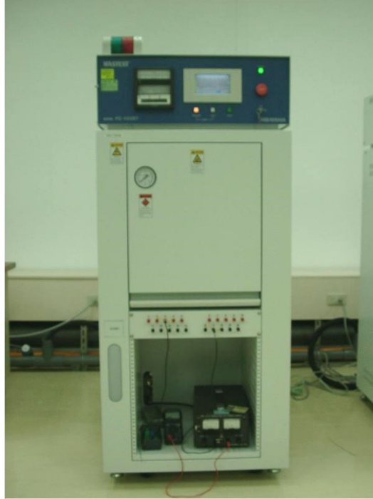
Figure 3. HIRAYAMA Pressure Oven, for HAST test
