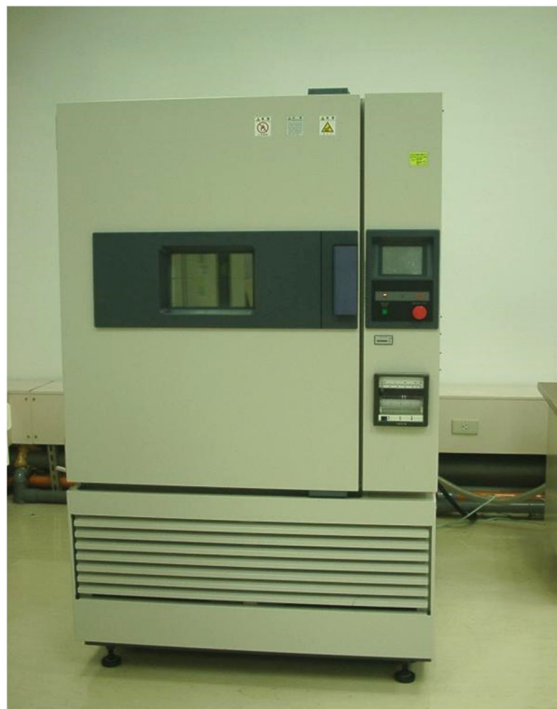
Figure 6. HITACHI Humidity Oven, for THS test
