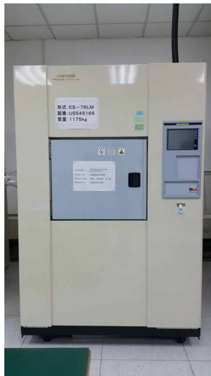
Figure 4. HITACHI Thermal Shock chamber for TCT test
