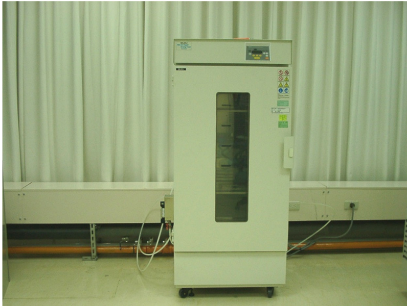
Figure 5. ISUZU High Temp Oven, for HTS test
