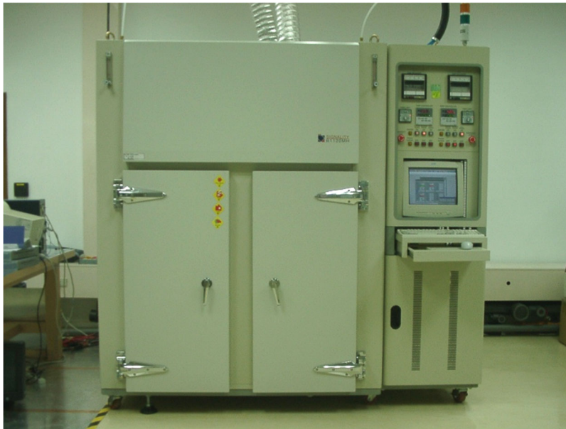
Figure 2. Signality Burn-in Oven, for HTOL test
