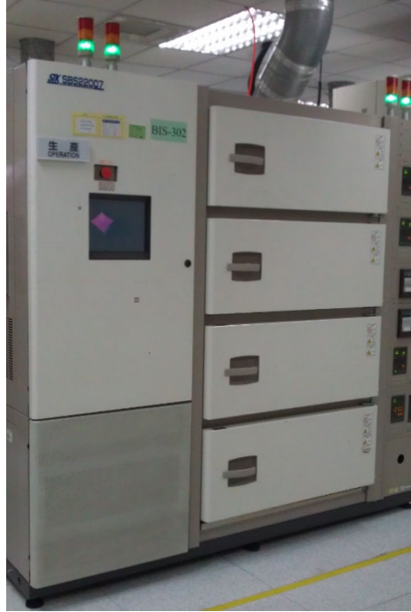
Figure 1. STK Burn-in Oven, for HTOL test
