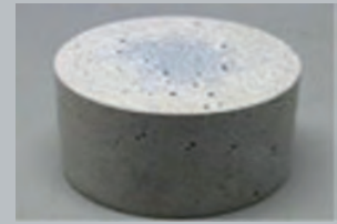
Figure 2 c: Set concrete following testing. The pores formed by escaping gas bubbles can be seen on the surface of the material. This sort of porosity is to be avoided as it means a reduction in quality.
