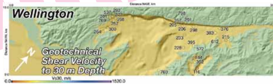
Figure 1: Map of average shear velocity from the surface to 30 m depth assembled for the Wellington – Lower Hutt region of New Zealand, with the 1500 m/s velocity isosurface in shaded relief to show bedrock and basin-floor topography from Benites and Olsen (2005). Locations of 27 of 46 sites measured in 2006 for shallow shear velocity are marked with dashed circles, labeled with the measured V_{s30} in m/s. Kaiser and Louie (2006) made an additional 19 measurements in one neighborhood in the lower center of the map, with only two results shown here. The measurements allowed a revision of the shallow velocity model, with V_{s30} not exceeding 800 m/s. The basin-bounding Wellington fault runs along the northwest side of the basin.
