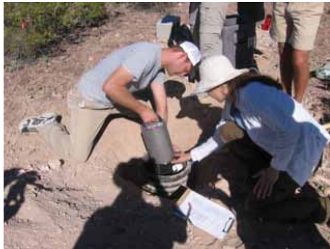
IRIS Interns installing a broadband seismic station in 2010. Students installed three stations and analyzed teleseismic seismograms recorded over a three-day period.
