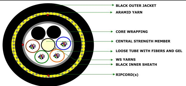
Typical construction Diagram - Not to Scale
