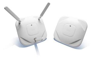
The new Cisco Aironet® 1600 Series Access Point is an enterprise-class, entry-level, 802.11n-based access point designed to address the wireless connectivity needs of small and medium-sized enterprise networks.
