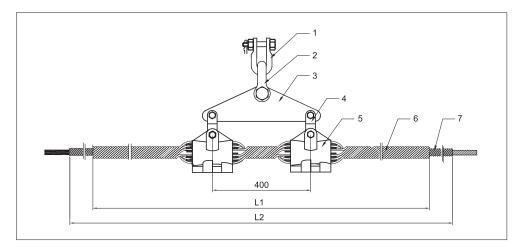
1. U shackle: Galvanized steel 2. Yoke plate: Galvanized steel
