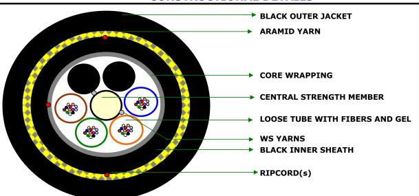
$\label{thm:construction} \mbox{ Typical construction Diagram - Not to Scale }$
