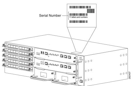
Figure iv-18 Cisco ASR 903 Router Serial Number Location
