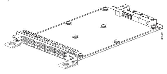
Figure iv-14 Cisco ASR 903 Router Front Panel
