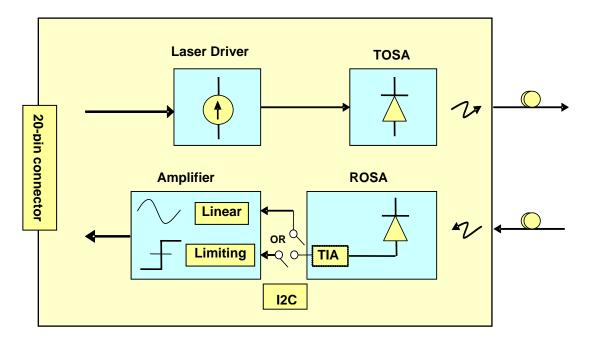
The block diagram shows two different SFP+ module implementations, one based on linear and one based on limiting receiver
