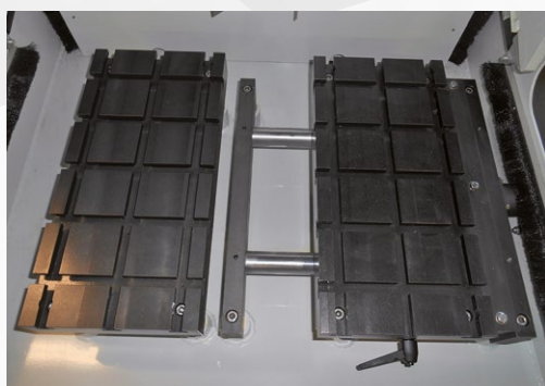
Transversal table X axis 120 mm stroke
