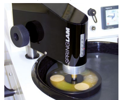
SPRINGLAM® pressure arm for SMARTLAM®2.0
