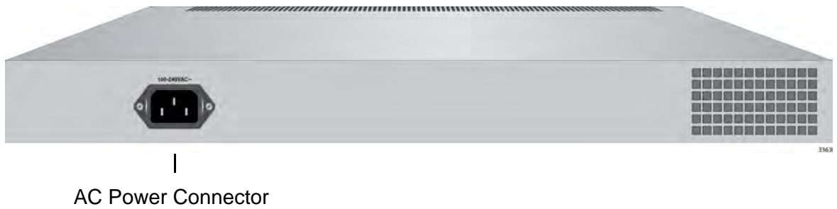
Figure 4. Back Panel of the AT-GS924MPX and AT-GS948MPX Switches
