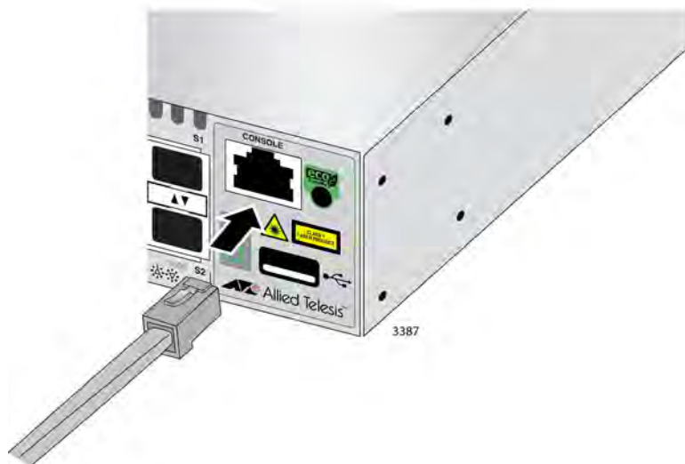
Figure 52. Connecting the Management Cable to the Console Port
