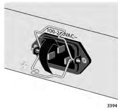
Figure 46. Raising the Retaining Clip
