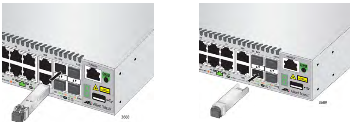
Figure 41. Installing an SFP Transceiver
