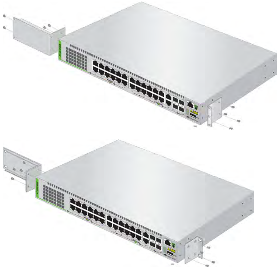
Figure 19. Installing Brackets on the AT-GS924MX Switch
