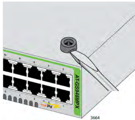
Figure 18. Removing the Rubber Feet
