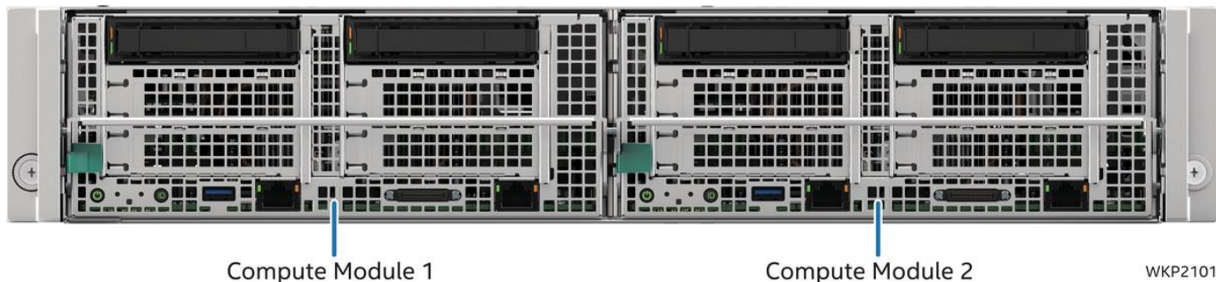
Figure 4. Compute module identification – two-node systems using 2U compute modules
