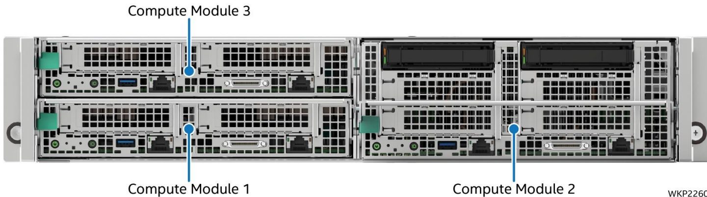
Figure 5. Compute module identification – mixed-node systems using two 1U and one 2U compute modules
