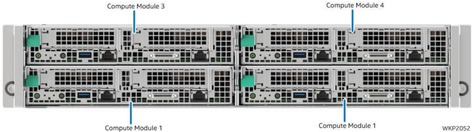
Figure 2. Compute module identification – systems with four 1U compute modules
