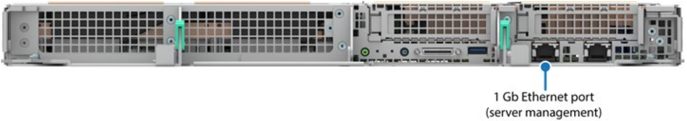
Figure 96. Dedicated Management Port – 1U Intel® Data Center GPU Max Series Accelerator Module
