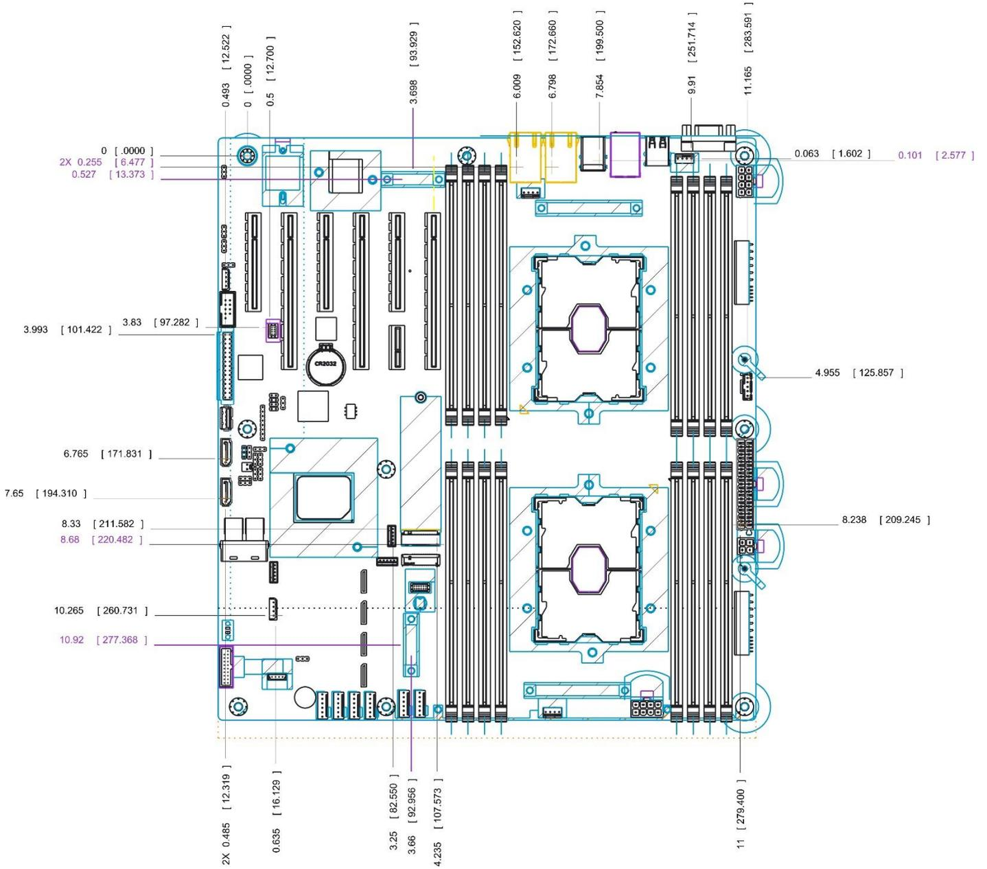
Figure 13. Major components and connectors (3 of 3)
