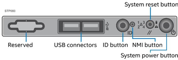
**Figure 53. Intel® Server Chassis P4304XXMFEN2/P4304XXMUXX front panel**
