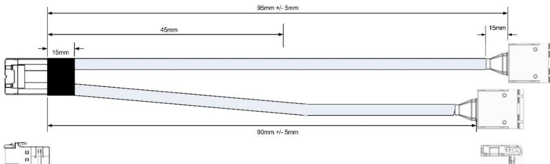
**Figure 27. Intel® QuickAssist Technology bridge cable – iPC AXXSTCBLQAT**
