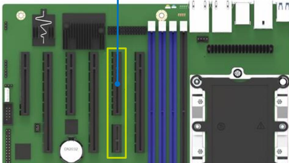
**Figure 40. SFP+ LAN Riser Option Support**
