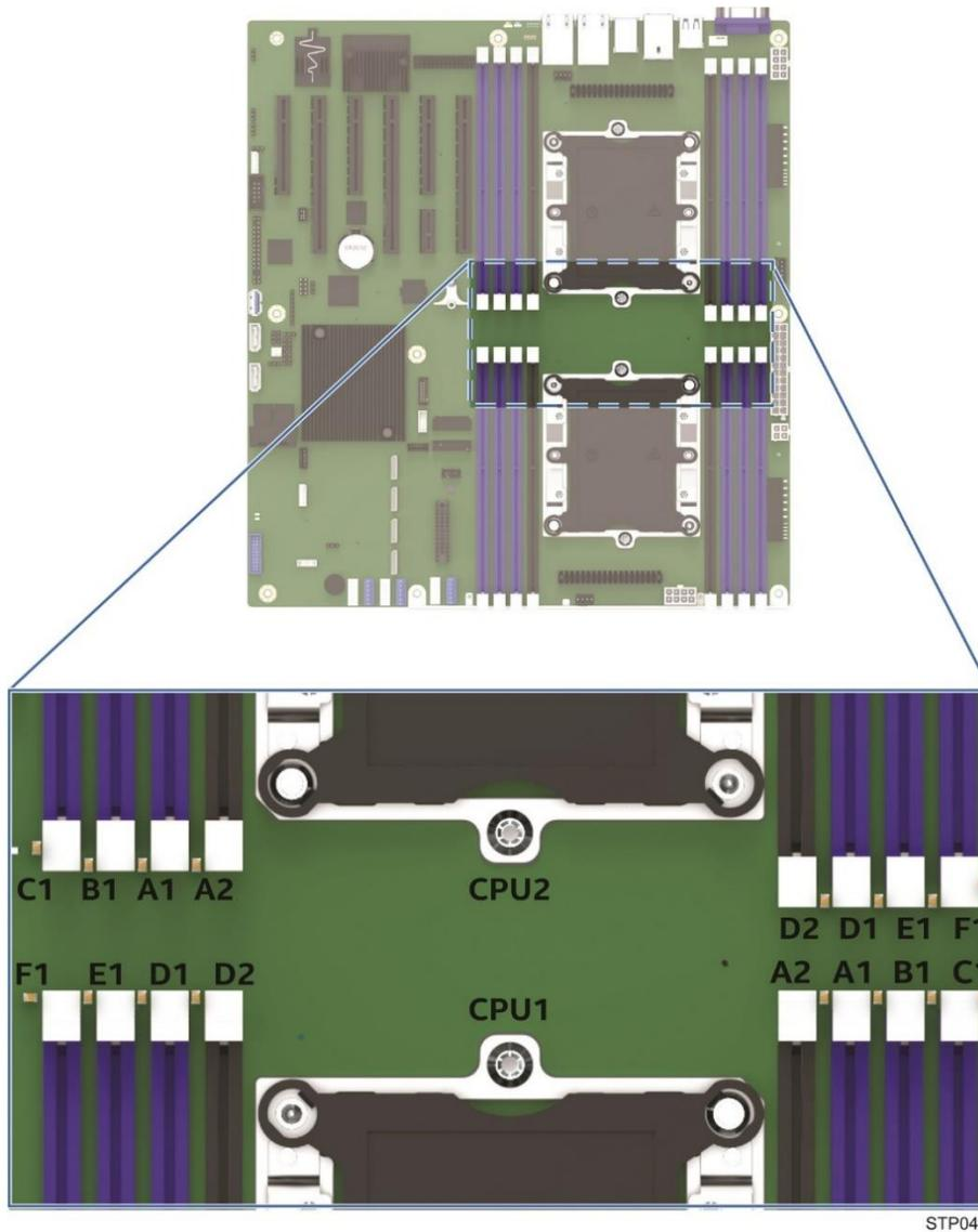
Figure 4. Intel® Light Guided Diagnostics - DIMM fault LEDs
