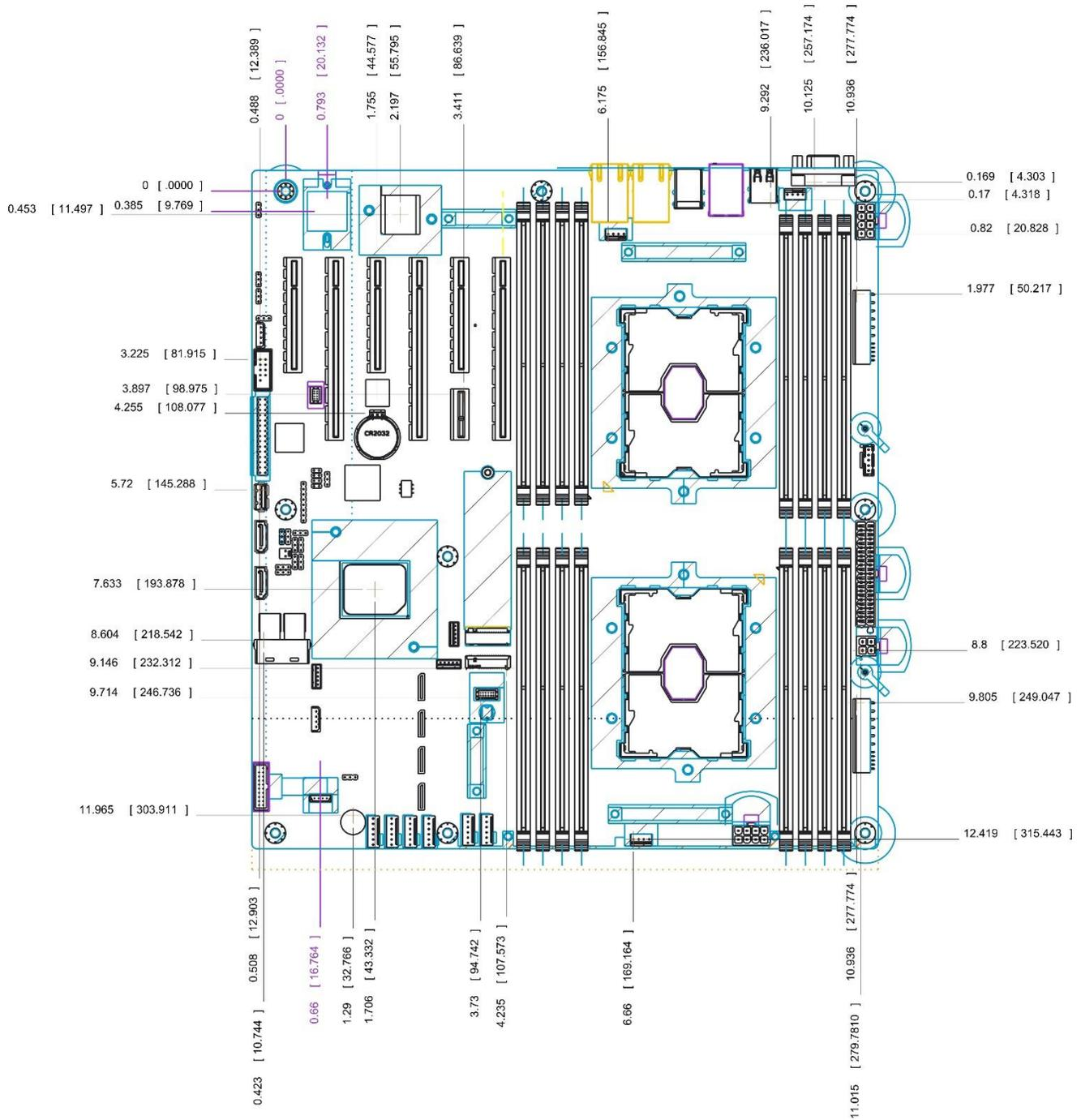
Figure 12. Major components and connectors (2 of 3)
