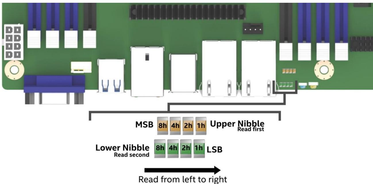
Figure 49. POST diagnostic LED location and definition
