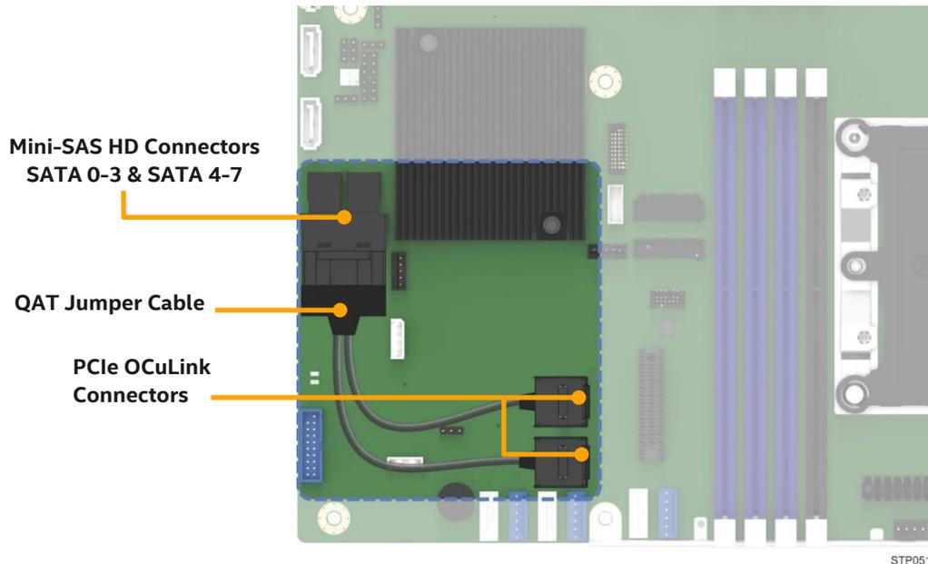
**Figure 26. Optional Intel® QuickAssist Technology bridge cable installed**
