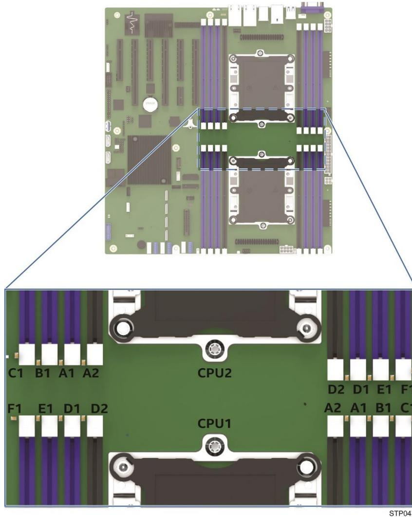
Figure 47. DIMM fault LEDs
