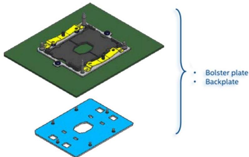
**Figure 16. Processor socket assembly**
