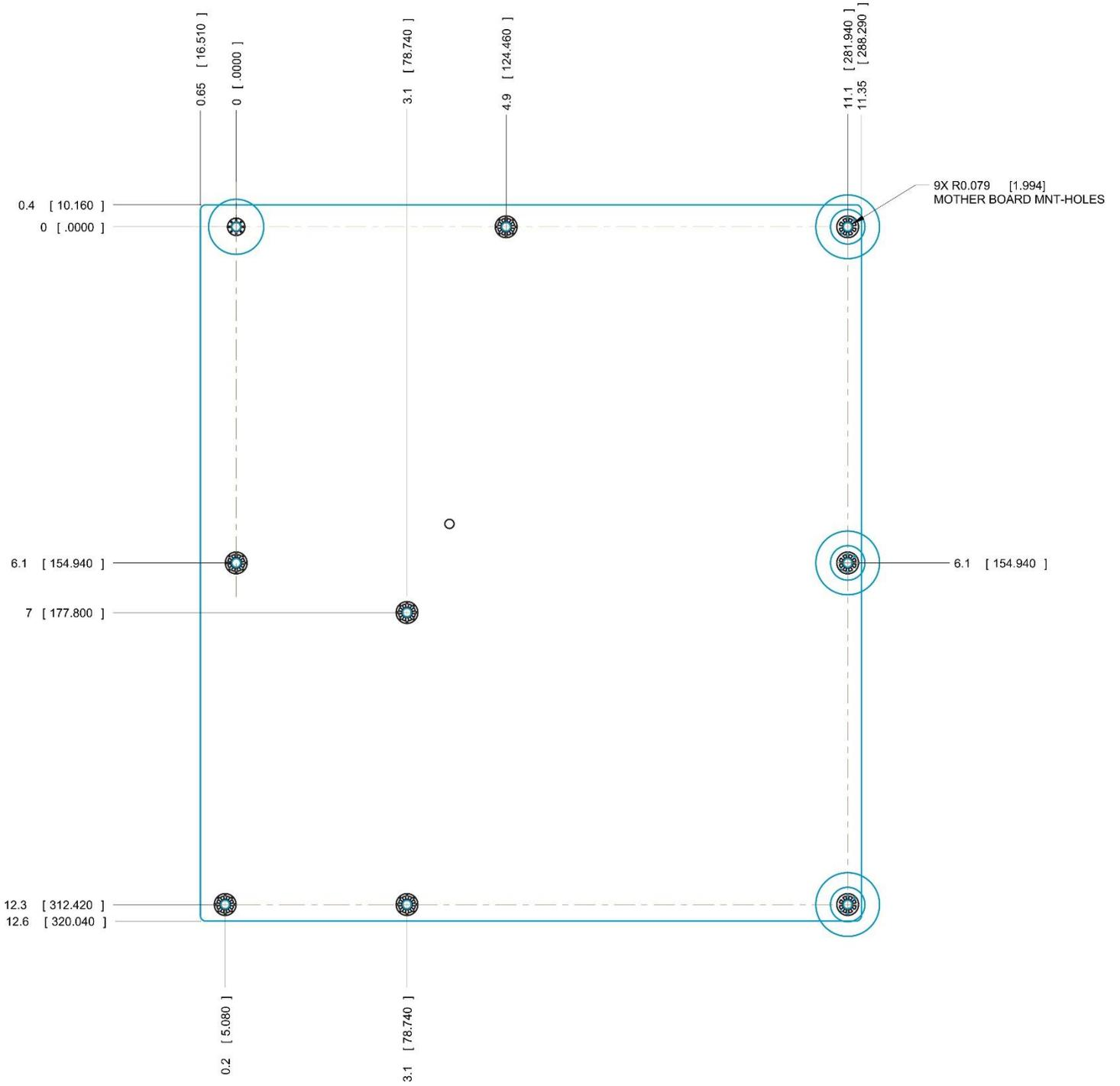
Figure 9. Mounting holes
