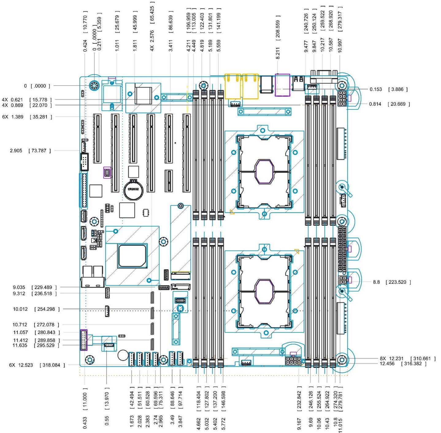
Figure 11. Major components and connectors (1 of 3)
