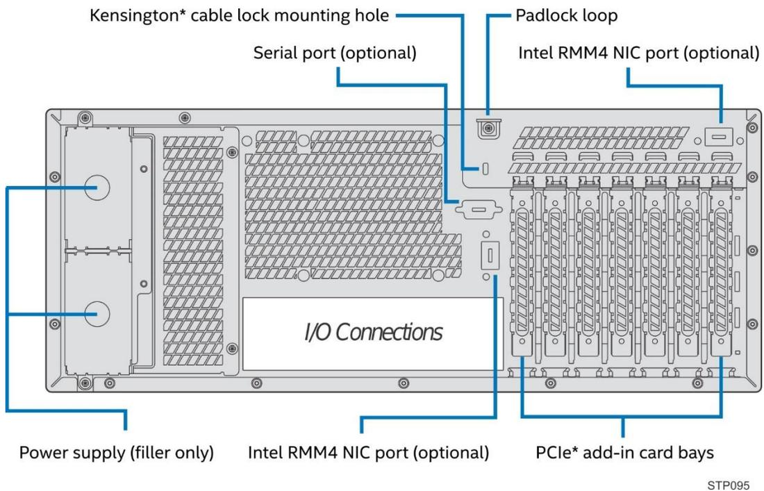
**Figure 55. Intel® Server Chassis P4304XXMUXX back panel**
