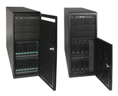
Figure 57. 2.5" and 3.5" storage configurations
